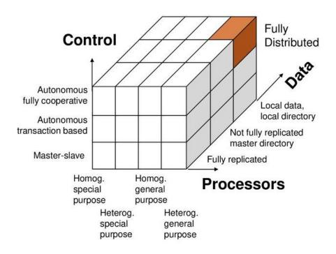
In a distributed system, hardware resources like processing power, storage, and network bandwidth are spread across multiple interconnected nodes, allowing for data and control to be distributed as well. This design enables parallel processing, enhances resilience, and facilitates resource sharing across different locations and devices.
