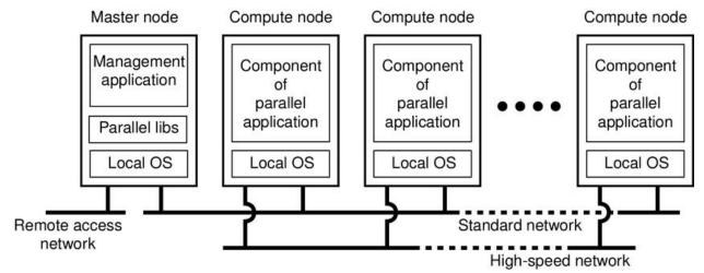
Each cluster consists of a collection of compute nodes that are controlled and accessed by means of a single master node. The master handles the allocation of nodes to a particular parallel program, maintains a batch queue of submitted jobs and provides an interface for the users of system as such the master actually runs the middleware needed for the exhibition of program and management of the cluster.
